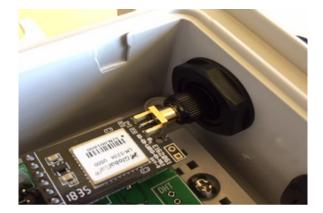
Connect the Watermark soil moisture sensors to wire terminals 1-4. Insert the battery connector to start the system
